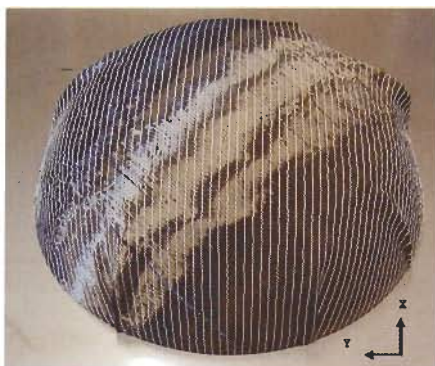
Fig. 2 Untreated fabric with threads with 6 folds at high diameters and draping heights
