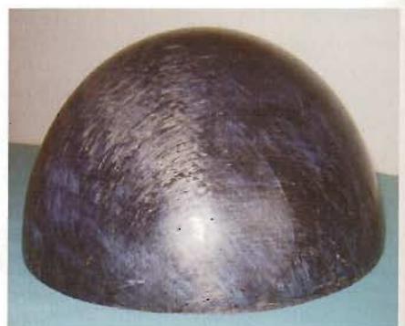
Fig. 4 Fiber composite (negative form - concave) with fold-free exterior, hemisphere diameter 298 mm, height 149 mm; hand laminate with epoxy matrix L20 and hardener EPH 161 with 4 layers of pre-draped multi-axial non crimp fabric
