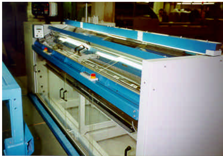
Fig. 2: View with partial capsuling in the front operating passage
