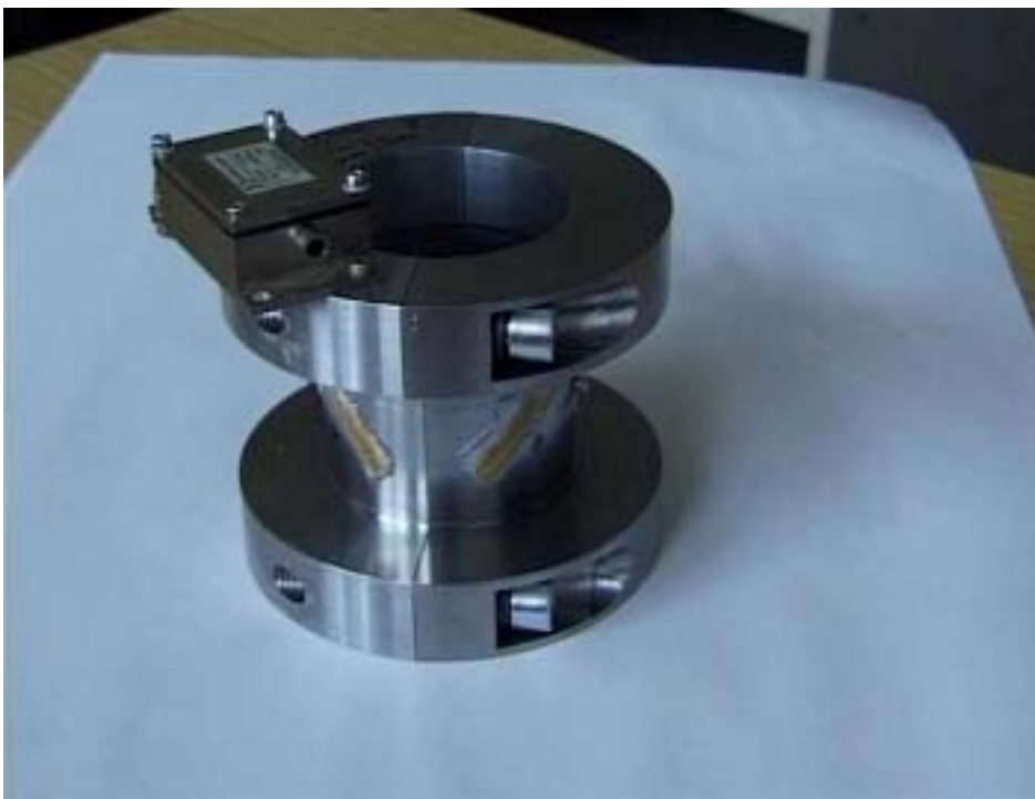
Figure 2: Thin-walled divided measurement hub for the contact-free measurement of the torque of the take-off roller
