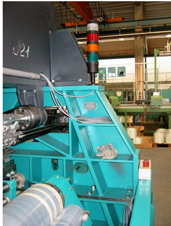
right frame wall with mineral molding
