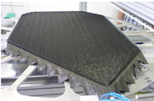
Near-Net-Shape-Versuchsanlage/Near net shape test facility
