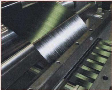
These UD tapes are suitable for use in various applications. On this basis, new structures can be manufactured on multiaxial machines with better quality and higher productivity. Good drapability, high energy absorption capacity and improved impact behaviour are some benefits of sewn multiaxial fabrics when compared with prepregs.
