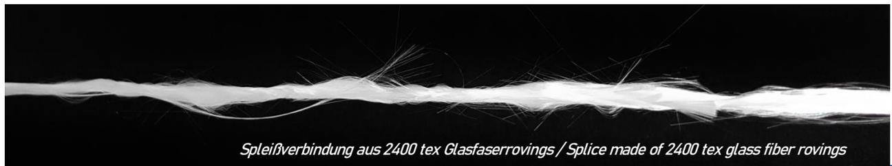
Spleißverbindung aus 2400 tex Glasfaserrovings / Splice made of 2400 tex glass fiber rovings
